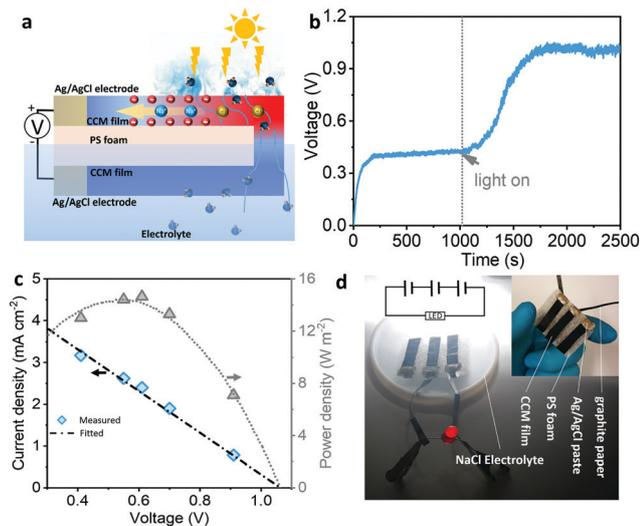
**Fig. 5** Proof-of-concept design for a solar power generation device. (a) Schematic of the device. (b) Measured open-circuit voltage of the device over time with and without light illumination. (c) Current density–voltage curve and calculated power density of the device under one sun illumination. (d) Photo of a red LED powered by a series of devices under one sun illumination. CCM = cellulose nanofibre @ conductive metal–organic framework; PS = polystyrene.
