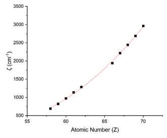
Fig. 4 CASSCF-SO-calculated SO coupling parameters (points) for trivalent lanthanide ions. Note here that the configuration  $4f^n$  is changing with Z as all ions are trivalent. Line is best fit with parameters in Table S7.†
