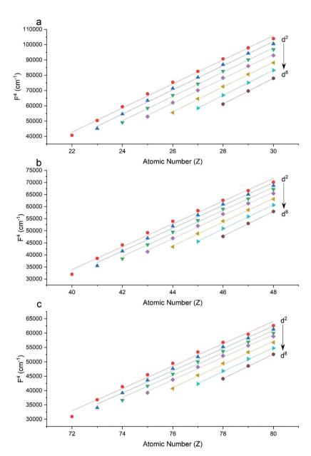
Fig. 3 CASSCF-SO-calculated F<sup>4</sup> parameters (points) for free ions (a) 3d, (b) 4d, (c) 5d. Lines are second-order polynomial fits, with parameters given in Table S6.†
