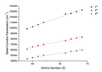
**Fig. 5** CASSCF-SO-calculated Slater—Condon ( $F^2$ ,  $F^4$ ,  $F^6$ ) parameters (points) for trivalent lanthanide ions. Note here that the configuration  $4f^n$  is changing with Z as all ions are trivalent. Lines are best fits with parameters in Table S7.†
