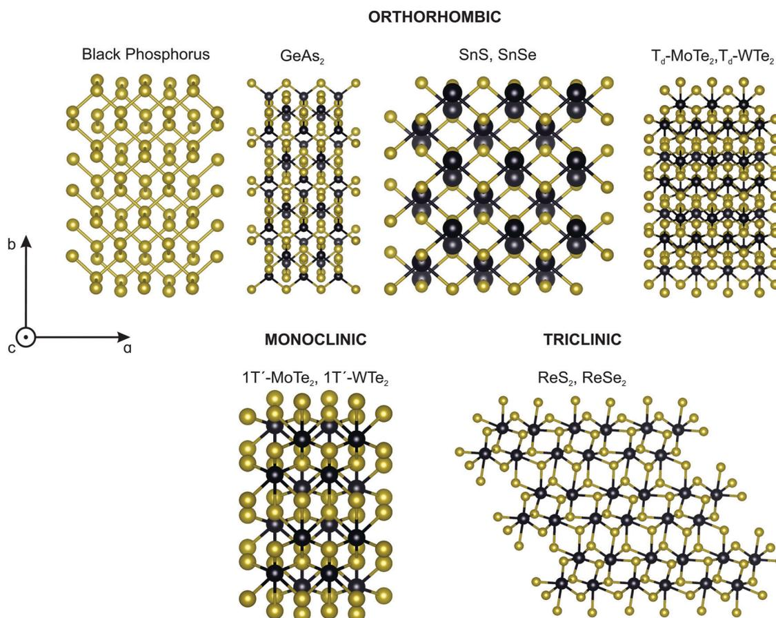
Fig. 3 Classes of low-symmetry 2D materials. Crystalline structure of the low-symmetry 2D materials: orthorhombic (e.g. back phosphorus, GeAs<sub>2</sub>, SnS, SnSe, T<sub>d</sub>-MoTe<sub>2</sub>, T<sub>d</sub>-WTe<sub>2</sub>), monoclinic (e.g. 1T'-MoTe<sub>2</sub>, 1T'-WTe<sub>2</sub>) and triclinic (ReS<sub>2</sub>, ReSe<sub>2</sub>).
