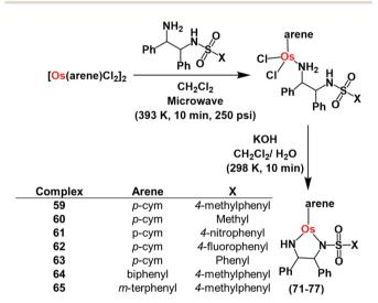
Fig. 16 Synthetic route for Os<sup>II</sup> arene sulfonamidoethylenediamine catalysts 59-65 for pyruvate reduction.
