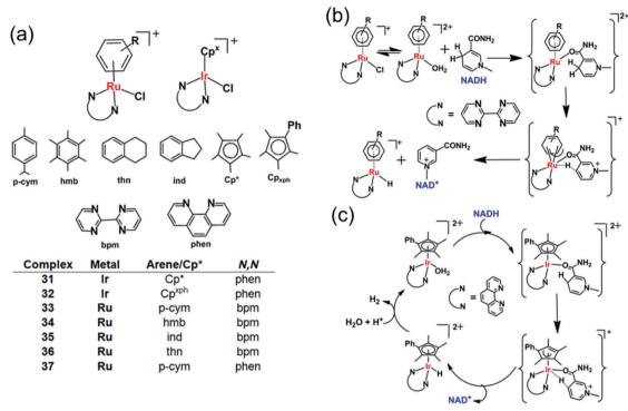
Fig. 11 Cyclopentadienyl Ir<sup>III</sup> (31, 32) and arene Ru<sup>II</sup> transfer hydrogenation catalysts (33–37) for NADH oxidation.<sup>26</sup> Proposed mechanism for transfer of hydride from 1,4-NADH to (b)  $Ru^{\parallel}$  and (c)  $Ir^{\parallel}$  complexes involving nicotinamide carbonyl coordination and arene/Cp ring slippage. <sup>26</sup>
