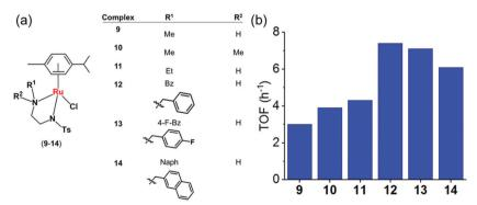
Fig. 6 (a) Structures of sulfonamidoethylenediamine  $Ru^{II}$  transfer hydrogenation catalysts **9–14**. <sup>22</sup> (b) Turnover frequencies (TOF) for reduction of NAD<sup>+</sup> by formate catalyzed by complexes **9–14**, determined by UV-vis spectroscopy (84 μM complex in MeOH/H<sub>2</sub>O 1:9 v/v, 102 mM sodium formate and 510 μM NAD<sup>+</sup> in H<sub>2</sub>O). <sup>22</sup>
