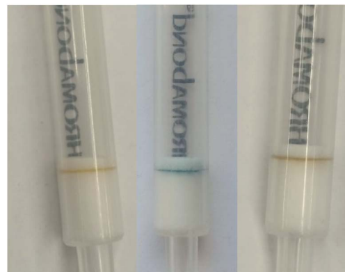
Fig. 7 Immobilizations of PV and Cu 2 II -PV on the top of C18ec cartridges at pH 6.50 ([HEPES] = 10 mM). Left: PV (2 mL, 5 μM; 10 nmol; dark yellow), middle: Cu 2 II -PV (2 mL, 5 μM; 10 nmol; detection zone: blue), right: Cu 2 II -PV + GlyP (2 mL, 5 μM, 10 nmol; detection zone: dark yellow).
