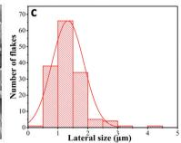
Fig. 1 (a) and (b) SEM images of GNP flakes; (c) Histogram of the lateral flake size for the GNP ink after 70 cycles of microfluidic exfoliation.
