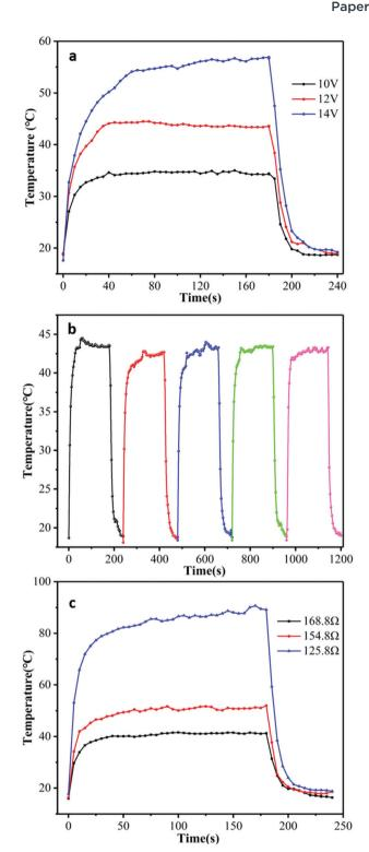
Fig. 4 (a) Temperature profiles of the GNP fabric at different  $V_{\text{GNP}}$ ; (b) temperature response of the GNP fabric over 5 cycles at  $V_{\rm GNP}$  = 12 V, each cycles is 4 min long; (c) temperature profiles of the GNP fabric operated at different biases.
