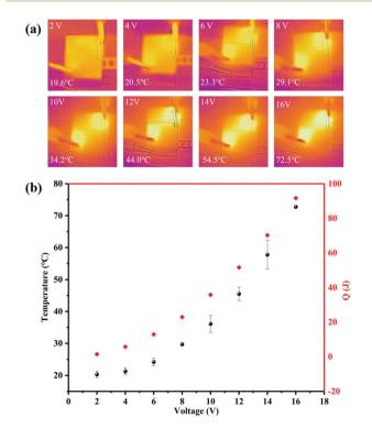
Fig. 3 (a) Infrared thermal images of the conductive fabric at various  $V_{\text{GNP}}$ ; (b) plot of the temperature versus  $V_{\text{GNP}}$ .
