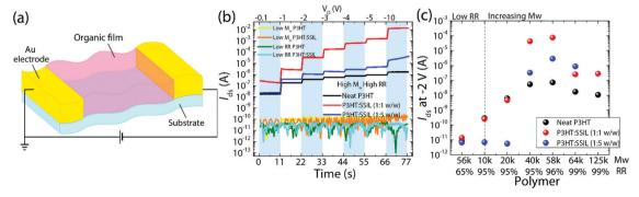
Fig. 2 (a) Diagram of the chemiresistor device structure; (b) driven voltage dependence across the  $L = 5 \mu m$  and W = 2 mm chemiresistor channel and (c) mean drain current measured for each polymer under an applied bias of  $V_D = -2 \text{ V}$ .
