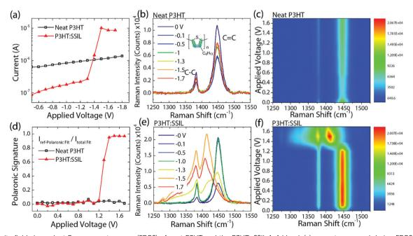
Fig. 5 In situ field-dependent Raman spectroscopy (FDRS) of neat P3HT and the P3HT: SSIL 1:1 blend. (a) current measured during FDRS. FDRS for (b) neat P3HT and (e) the P3HT: SSIL blend. 2D Raman intensity plot at different applied voltages for (c) neat P3HT and (f) the P3HT: SSIL blend. (d) Polaronic signature fitted by a linear combination of the reference neutral and polaronic P3HT Raman peaks.
