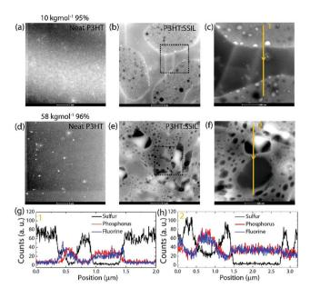
Fig. 3 HAADF-STEM images of P3HT neat and P3HT:SSIL 1:1 films: low  $M_{\rm w}$  P3HT (a) neat and (b) blend, and high  $M_{\rm w}$  P3HT (d) neat and (e) blend (scale bar:  $1 \mu m$ ). 1-D elemental profile on the selected region of the low  $M_{\rm w}$  blend ((1) c and g) and the high  $M_{\rm w}$  blend ((2) f and h).
