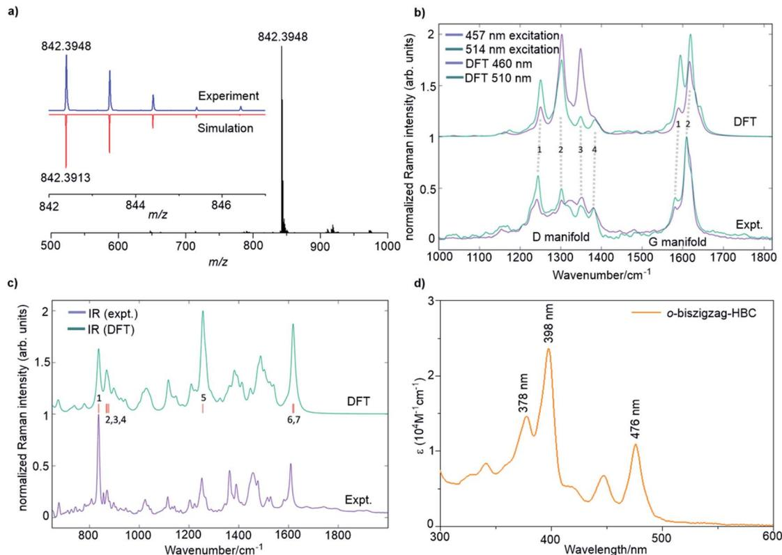
**Fig. 2** (a) MALDI-TOF MS of **4**. Inset: isotopic distribution compared with the mass spectrum simulated for C<sub>66</sub>H<sub>50</sub>. (b) FT-Raman spectra of **4** compared with results from DFT calculations over the D and G regions. (c) Micro FT-IR spectrum of **4** and the simulated spectrum by DFT calculations. (d) UV/vis absorption spectrum **4** in THF. Concentration: 2 × 10<sup>−5</sup> M.
