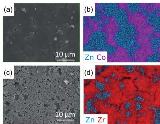
Fig. 3 Surface morphology and elemental distribution of CGCs. SEM images and EDS maps of metal centres on the surface of CGCs (a and b)  $(\text{ZIF-67})_{0.5}(\text{a}_9\text{ZIF-62})_{0.5}$  and (c and d)  $(\text{UiO-66})_{0.5}(\text{a}_9\text{ZIF-62})_{0.5}$ .
