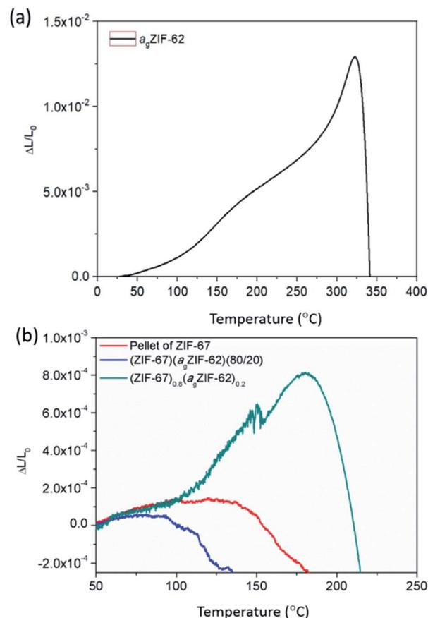
Fig. 6 Thermo-mechanical properties. Linear thermal expansion of (a) a<sub>g</sub>ZIF-62 and (b) ZIF-67 series measured by TMA.
