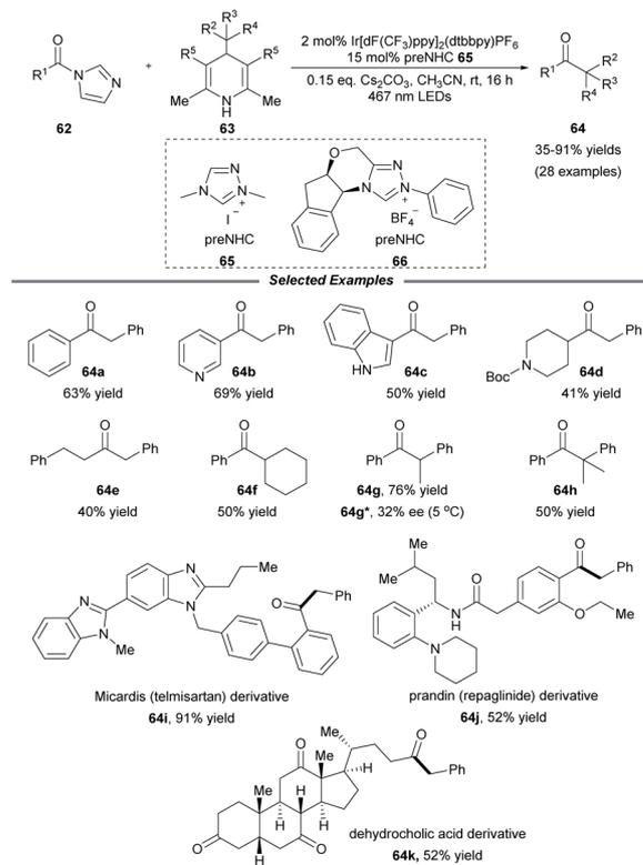
**Scheme 7** Alkylation of acyl azoliums for the synthesis of ketones. dF(CF<sub>3</sub>)ppy: 2-(2,4-difluorophenyl)-5-trifluoromethylpyridine.
