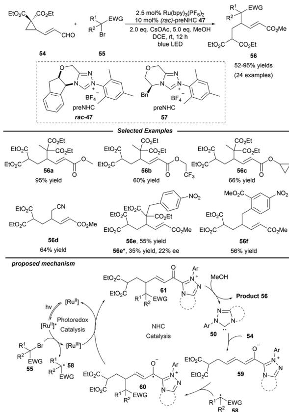
the product **56e** in a promising enantioselectivity with 22% ee. Mechanistically, NHC **50** reacts with  $\gamma$ -cyclopropane enal **54** to give the dienolate intermediate **59**, which can be trapped by radical **58** which is generated from the alkyl halide *via* photoredox catalysis. The afforded homoenolate radical **60** undergoes a subsequent SET oxidation and alcoholysis to regenerate the NHC catalyst and provide the final product **56**.
