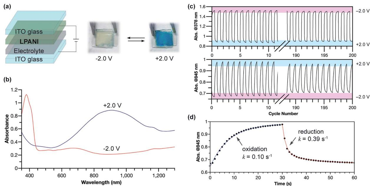
Fig. 6 (a) Architecture and photographic images of the electrochromic device at  $-2.0$  V and  $+2.0$  V, respectively. (b) Absorption spectra of the electrochromic device when applying  $-2.0$  V or  $+2.0$  V for 60 s. (c) Absorbance at 378 nm and 845 nm with voltage swept between  $-2.0$  V and  $+2.0$  V for 200 cycles. (d) Time-dependent absorbance changes at 845 nm; dots: experimental data spots; lines: pseudo-first-order fitting.
