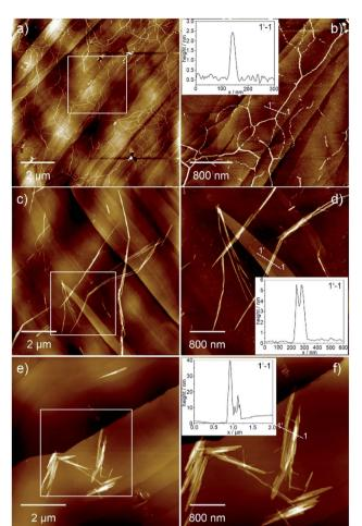
Fig. 3 AFM images of Agg I (a and b), Agg II (c and d) and Agg IIc superstructures (e and f) obtained upon spin-coating the corresponding solutions onto HOPG. The insets show the height profile along the 1-1' axis depicted in the images.
