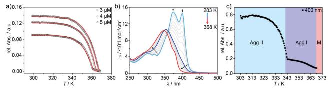
Fig. 5 (a) Aggregation curves of Agg I ( $\lambda=400$  nm) upon cooling hot monomer solutions from 368 K to 298 K and fits to the nucleation-elongation model. (b) UV-Vis spectra recorded upon heating Agg II under constant mechanical agitation ( $c=5\times10^{-6}$  M). (c) Corresponding two-stage disassembly curve recorded at  $\lambda=400$  nm.
