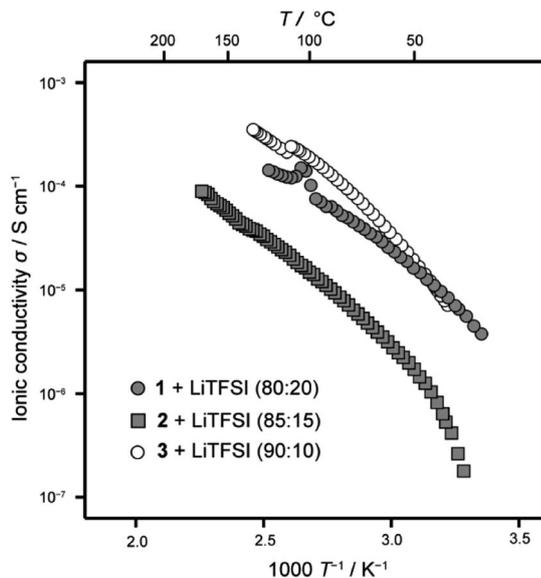
Fig. 6 Ionic conductivities of LC mixtures 1–3 with LiTFSI.
