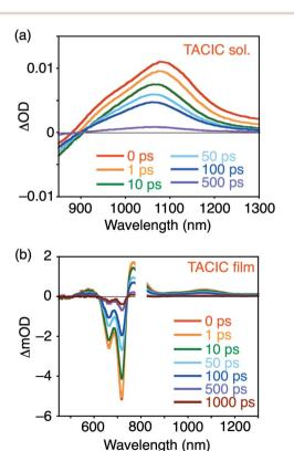
Fig. 3 Transient absorption spectra of (a) TACIC in chloroform in 0–500 ps and (b) TACIC film in 0–1000 ps. The excitation wavelength ( $\lambda_{ex}$ ) and intensity were (a) 650 nm and 26  $\mu J$  cm<sup>-2</sup> and (b) 700 nm and 0.68  $\mu J$  cm<sup>-2</sup>.
