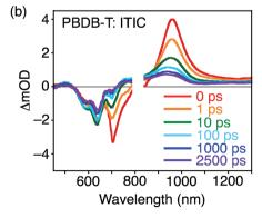
Fig. 5 Transient absorption spectra of (a) PBDB-T:TACIC and (b) PBDB-T:ITIC blend films measured from 0-2500 ps. The excitation wavelength and intensity were 700 nm and 7.5 μJ cm<sup>-2</sup>, respectively.
