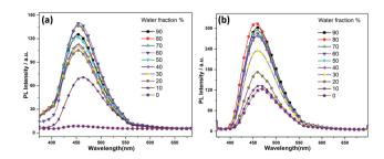
Fig. 3 Fluorescence spectra of (a)  $\bf 1$  and (b)  $\bf 2$  in water/THF mixture with the increases of the water fractions, starting from  $\bf 10-90\%$ .
