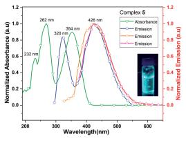
Fig. 9 UV/vis absorption (green line) and emission (blue, orange and red lines when excited at 262, 320 and 354 nm, respectively) spectra of complex 5 in MeCN solution.
