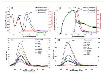
Fig. 1 (a) UV-visible absorption (left) and emission spectra (right) of 1 and 2 in DCM; (b) solid-state DRS-UV (left) and emission spectra (right) of 1 and 2; (c) PL spectra of 1 (left); (d) PL spectra of 2 (right) in different solvents.
