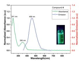
Fig. 10 UV/vis absorption and emission spectra of Me<sub>3</sub>CpK(THF) (4).
