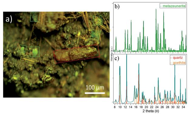
Fig. 3 Microphotograph of the surface: green crystals of metazeunerite, dark-brown quartz, and light-brown, needle-shaped goethite crystals (a); u-PXRD patterns of green crystals selected from the surface of the granitic rock and database metazeunerite (ICDD – 40148463) (b); and light- and dark-brown crystals correspond to goethite (ICDD - 290713) and guartz (ICDD - 0898935), respectively (c).
