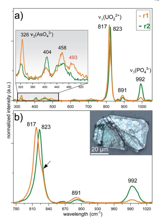
Fig. 4 Raman spectra of two different green crystals selected from the surface ('r1', analysed by μ-PXRD corresponds to metazeunerite) and from the cavity ('r2') of the rock with zoomed 290–550 cm $^{-1}$  region (a); Raman spectra for the 780–1020 cm $^{-1}$  region. Image of the  $\sim$ 50  $\mu$ m size flat-shaped microcrystal selected from rock's cavity done with Raman spectrometer for 'r2'. Arrow indicates on the spectral feature in 'r1' presumably referring to U-phosphate phase (b).
