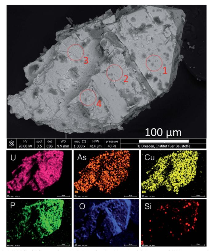
Fig. 5 SEM-EDX analysis for a green microcrystal selected from the surface of the granite rock. Dark grey areas on the SEM image correspond to Fe from the goethite debris. Red dotted circles show the spots at which EDX measurements were performed (Table 1).
