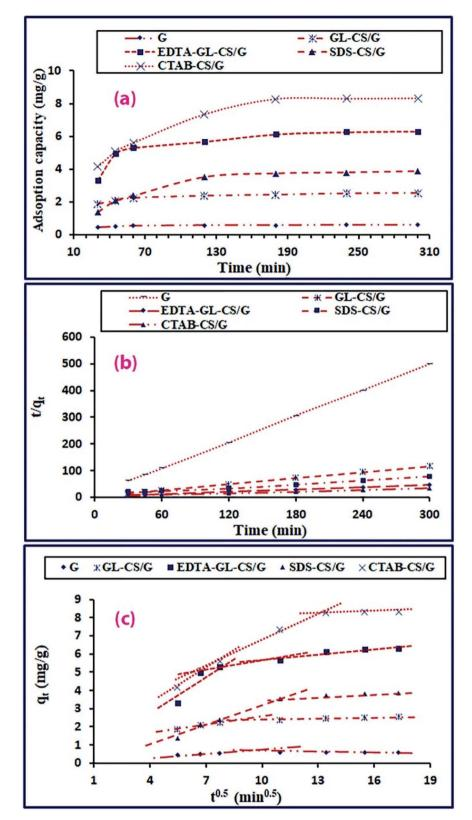
Fig. 6 Effect of contact time (a), and the pseudo-second-order kinetic model (b), and validation of intra-particle diffusion model (c) for F<sup>-</sup> ions adsorption on G, GL-CS/G, EDTA-GL-CS/G, SDS-CS/G and CTAB-CS/G adsorbents.
