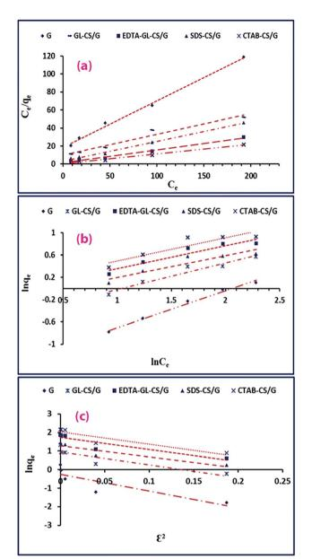
Fig. 7 Langmuir isotherm (a), Freundlich isotherm (b), and Dubinin–Radushkevich isotherm (c) models for the  $F^-$  ions adsorption on G, GL-CS/G, EDTA-GL-CS/G, SDS-CS/G and CTAB-CS/G adsorbents.
