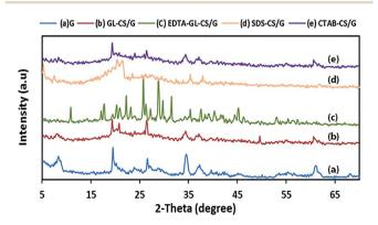
Fig. 1 XRD patterns of G (a), GL-CS/G (b), EDTA-GL-CS/G (c), SDS-CS/G (d), and CTAB-CS/G (e) products.
