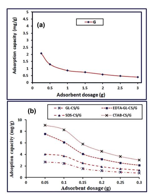
Effect of adsorbent dosage on the F<sup>-</sup> ions adsorption on G (a); GL-CS/G, EDTA-GL-CS/G, SDS-CS/G, and CTAB-CS/G (b) adsorbents.
