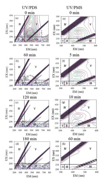
Fig. 6 3D-EEM spectra of HA at various reaction times in UV/PDS (a–d) and UV/PMS (e–h). Conditions:  $[HA]_0=15~mg~L^{-1}$ ,  $[PDS]_0=3~mmol~L^{-1}$ ,  $[PMS]_0=1~mmol~L^{-1}$ ,  $pH_0=6~and~3~for~UV/PDS~and~UV/PMS$ , respectively.
