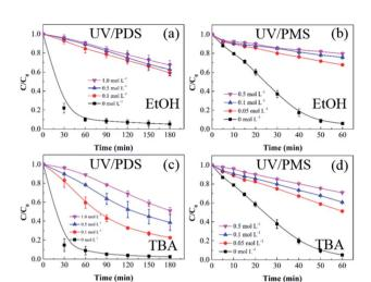
Fig. 4 Effects of radical scavengers on HA removal in UV/PDS (a and c) and UV/PMS (b and d). Conditions:  $[HA]_0=15~mg~L^{-1}$ ,  $[PDS]_0=3~mmol~L^{-1}$ ,  $[PMS]_0=1~mmol~L^{-1}$ ,  $pH_0=6~and~3~for~UV/PDS~and~UV/PMS$ , respectively.
