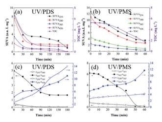
Fig. 5 Evolution of the SUVA and UV spectroscopic ratios during HA removal in UV/PDS (a and c) and UVPMS (b and d). Conditions: [HA] $_0$  = 15 mg L $^{-1}$ , [PDS] $_0$  = 3 mmol L $^{-1}$ , [PMS] $_0$  = 1 mmol L $^{-1}$ , pH $_0$  = 6 and 3 for UV/PDS and UV/PMS, respectively.
