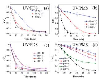
Fig. 3 Effects of the initial HA amount on HA removal in UV/PDS (a) and UV/PMS (b). Conditions:  $[HA]_0 = 5-45 \text{ mg L}^{-1}$ ,  $[PDS]_0 = 3 \text{ mmol L}^{-1}$ ,  $[PMS]_0 = 1 \text{ mmol L}^{-1}$ ,  $pH_0 = 6 \text{ and } 3 \text{ for UV/PDS and UV/PMS, respectively. Effects of the initial solution pH on HA removal in UV/PDS (c) and UV/PMS (d). Conditions: <math>[HA]_0 = 15 \text{ mg L}^{-1}$ ,  $[PDS]_0 = 3 \text{ mmol L}^{-1}$ ,  $[PMS]_0 = 1 \text{ mmol L}^{-1}$ ,  $pH_0 = 3-11$ .
