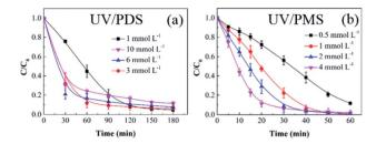
Fig. 2 Effects of the oxidant dose on HA removal in UV/PDS (a) and UV/PMS (b). Conditions:  $[HA]_0=15~mg~L^{-1}$ ,  $[PDS]_0=1-10~mmol~L^{-1}$ ,  $[PMS]_0=0.5-4~mmol~L^{-1}$ ,  $pH_0=6~and~3~for~UV/PDS~and~UV/PMS$ , respectively.
