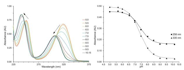
Fig. 1 Left: the UV-Vis absorption spectrum of Eu(iii)-DO3A-HMP (100  $\mu$ M, 0.1 M NaCl) hypsochromically shifts with increasing pH, consistent with deprotonation and attributed to greater electron density on the coordinating oxygen. Right: least squares fitting of absorption maxima (258 and 335 nm) vs. pH yields a p $K_a$  of 7.4.
