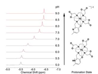
Fig. 3 The chemical shift of the resonance of Yb-DO3A-HMP varies in concert with UV-Vis and luminescent changes across the range of pH 6 to pH 8 due to induced changes in the Yb( $\bowtie$ ) dipolar field by changing HMP coordination upon deprotonation.
