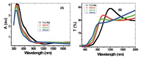
Fig. 4 Optical (A) absorbance (B) transmittance of pure and Cr-doped nanostructured PbS thin films.
