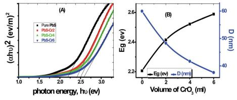
Fig. 5 (A) Plots of  $(\alpha h \nu)^2$  versus  $h\nu$  to determine  $E_q$  of pure and Cr-doped PbS films, (B) dependence of  $E_q$  and D on the level of Cr doping.
