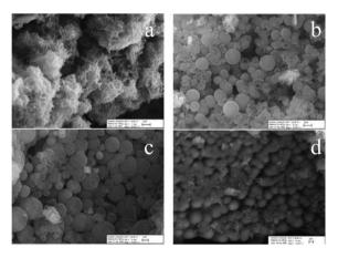
Fig. 22 SEM images of (a) PANI, (b) poly-2-fluoroaniline, (c) poly-2-chloroaniline, and (d) poly-2-methylaniline. Reproduced with permission from ref. 98.
