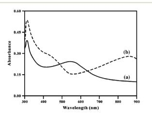
Fig. 14 Electronic spectrum of undoped (a) and doped (b) poly[bis(2-aminophenyloxy)disulfide] in DMF. Reproduced with permission from ref. 101.
