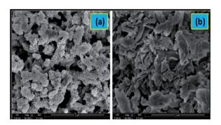
Fig. 23 SEM images of HCl-doped forms of (a) PANI, (b) poly-3-flu-oroanilline. Reproduced with permission from ref. 24.
