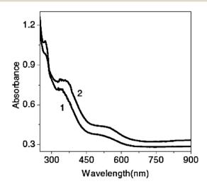
Fig. 15 Electronic spectra of polyanthranilic acid obtained by: 1 - single-phase method; 2 - two-phase method in 0.5 N H<sub>2</sub>SO<sub>4</sub>. Reproduced with permission from ref. 80.
