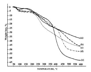
Fig. 18 Thermogravimetric curves of PANI (a), poly-2-fluoroaniline (b), poly-2-chloroaniline (c), poly-2-methylaniline (d) and poly-Nmethylaniline (e). Reproduced with permission from ref. 98.
