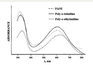
**Fig. 11** Electronic absorption spectrum of PANI derivatives in DMF. Reproduced with permission from ref. 70.
