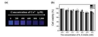
Fig. 9 (a) N,S-GQD-based paper strips for visual and rapid sensing and screening of Co<sup>2+</sup> under UV light irradiation of 365 nm. (b) Cellular toxicity determined by MTT assay with HeLa cells upon 24, 48, and 72 hours of incubation with different concentrations of N,S-GQDs from 0.0 to 3.0 mM.
