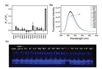
Fig. 5 (a) The degree of fluorescence quenching  $(F_0 - F/F_0)$  of 0.2 mM N,S-GQDs in the presence of 30  $\mu M$  Co<sup>2+</sup> and various other cations in 50 mM Tris-HCl buffer solution at pH 9.0. (b) The fluorescence emission spectra for the data in panel (a). (c) Photographs of the emission of 20 mM N,S-GQDs in the presence of 1 mM concentrations of various cations in 500 mM Tris-HCl buffer solution at pH 9.0 and under UV light irradiation of 365 nm
