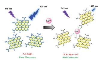
Fig. 7 Schematic representation of the complexation of Co<sup>2+</sup> and N.S-GQDs via metal-ligand interactions and accompanying fluorescence quenching.
