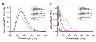
Fig. 3 (a) The normalized fluorescence emission spectra of 0.4 mM N,S-GQDs, 0.4 mM N,S-GQDs in the presence of 50 mM Tris-HCl buffer pH 9.0, and 0.4 mM N,S-GQDs in the presence of 50 mM Tris-HCl buffer pH 9.0 and 30  $\mu$ M Co<sup>2+</sup> compared with those of 0.4 mM cysteamine, 0.4 mM citric acid, and 30  $\mu$ M Co<sup>2+</sup> solutions under excitation wavelength at 345 nm. (b) The corresponding UV-Vis absorption spectra of panel (a).
