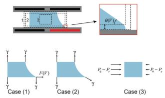
Fig. 4 Cross section of a droplet in a typical EWOD device with force analysis from different perspectives.
