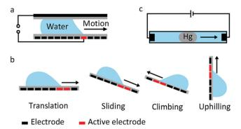
Fig. 5 Droplet transfer. (a) Water droplet transfer between two parallel electrode plates. (b) Water droplet sliding, climbing and uphilling on a coplanar electrode. (c) A mercury droplet immersed in saline is transferred towards the cathode.
