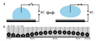
Fig. 9 Droplet bouncing. (a) A diagram of droplet bouncing under electric field. (b) A saline droplet with a volume of 8  $\mu L$  bouncing on a superhydrophobic substrate with an AC electric field of 100 V and 30 to 31 Hz.
