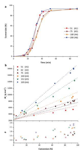
Fig. 5 PEG-X mediated VAc emulsion polymerizations when targeting different DPs for the PVAc block. Evolution of (a) conversion *versus* time and (b) number-average molar masses  $M_{\rm n}$  (plain squares) and dispersity ( $D = M_{\rm w}/M_{\rm n}$ , hollow squares) with VAc conversion (the dashed lines correspond to the theoretical  $M_{\rm n}$  values). See Table 1 for details.
