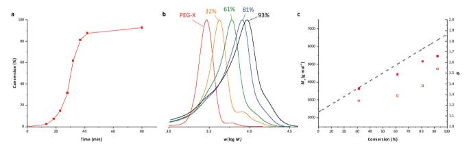
Fig. 1 PEG-X mediated VAc emulsion polymerization for DP<sub>target</sub> = 51 (entry A1, Table 1). (a) Evolution of conversion *versus* time, (b) SEC traces (RI detection) for samples withdrawn during the polymerization. (c) Corresponding evolution of the number-average molar masses  $M_n$  (plain squares) and dispersity ( $D = M_w/M_{nv}$ , hollow squares) with VAc conversion (the dashed line corresponds to the theoretical  $M_n$  values).
