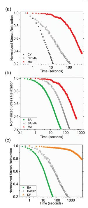
Fig. 5 Normalized stress relaxation data for (a) CY-Net, CY/MA-Net, and MA-Net; (b) BA-Net, BA/MA-Net, and MA-Net; (c) BA-Net, BA/DP-Net, and DP-Net at 140 °C.
