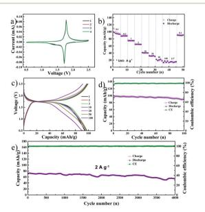
Fig. 3 (a) Results of CV tests conducted on the symmetric NVP cell in the DME electrolyte at a scan rate of 0.1 mV s $^{-1}$  in the 0.5 V to 2.5 V voltage window. (b) Results of rate performance tests conducted on the symmetric cell. (c) Voltage profile and (d) the corresponding cycling performance at a current density of 0.1 A g $^{-1}$ . (e) Cycling performance at a current density of 2 A g $^{-1}$ .
