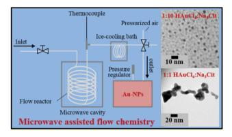
Fig. 8 Experimental setup for microwave assisted synthesis of gold nanoparticles. <sup>121</sup> This figure has been adapted/reproduced from ref. 121 with permission from the American Chemical Society, copyright 2016.
