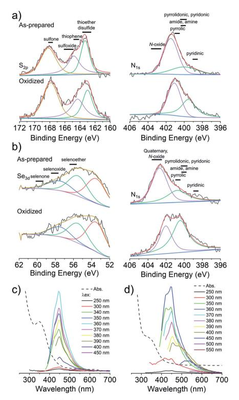
Fig. 3 CNDs produced from citric acid and  $C_2/Se-C_2$  are surface N-doped and core N, $S_{(0x)}/Se_{(0x)}$ -doped. High-resolution XPS spectra ( $S_{2p}$ ,  $N_{1s}$ ) before and after oxidation with  $H_2O_2$  of  $CND_{C_2}$  (a) and  $CND_{Se-C_2}$  (b). Spectral decomposition of the XPS spectra was performed to guide the eye. Absorbance and excitation-dependent fluorescence spectra of  $CND_{C_2}$  (c) and  $CND_{Se-C_2}$  (d).
