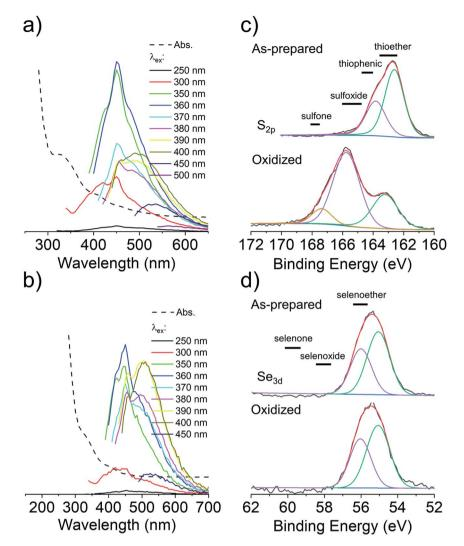
Fig. 4 CNDs produced from citric acid and M/Se-M are surface and core N,S/Se-doped. Absorbance and excitation-dependent fluorescence spectra of  $CND_M$  (a) and  $CND_{Se-M}$  (b). High-resolution XPS spectra ( $S_{2p}$ ,  $Se_{3d}$ ) before and after oxidation with  $H_2O_2$  of  $CND_M$  (c) and  $CND_{Se-M}$  (d). Spectral decomposition of the XPS spectra was performed to guide the eye.
