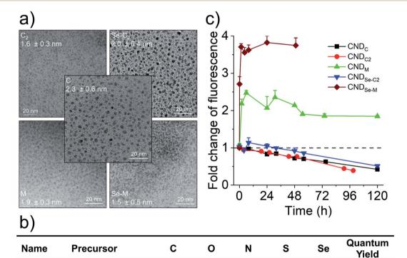
Fig. 1 Structure, composition, and optical characteristics of CNDs. (a) Representative TEM images of CNDs and average particle size. (b) Elemental composition of CNDs by XPS, and fluorescence quantum yield. (c) Evolution of fluorescence emission of CNDs ( $\lambda_{ex}$  360 nm;  $\lambda_{em}$  is the maximum emission wavelength seen in subsequent figures) in the presence of 50 mM  $H_2O_2$ . Data presented as mean + SD, n = 3.
