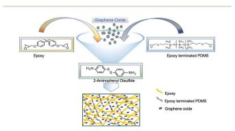
Fig. 1 Synthesis route of epoxy-PDMS-GO nanocomposite.
