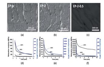
Fig. 3 (a) SEM image of EP-p. (b) SEM image of epoxy/PDMS. (c) TEM image of epoxy/PDMS/GO nanocomposite. Stress relaxation analysis at different temperatures for (d) EP-p, (e) EP-2 and (f) EP-2-0.5.
