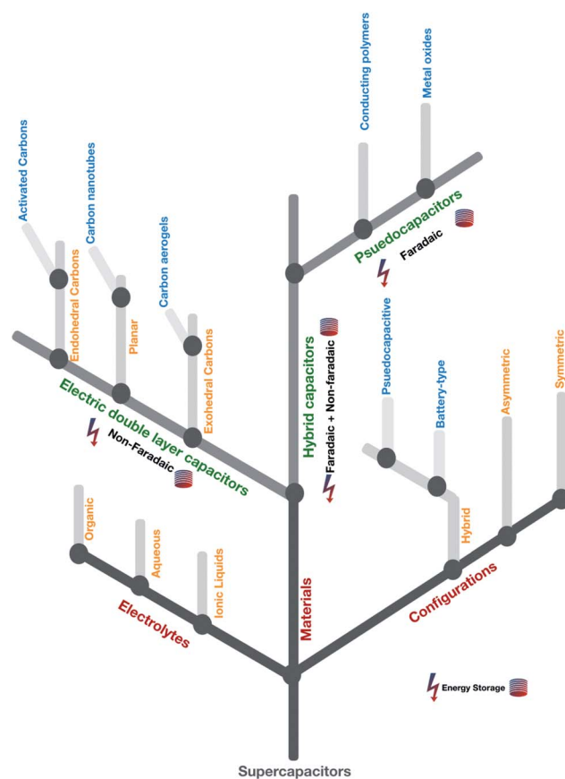
Fig. 2 An overview of the taxonomical classification of supercapacitors. The lightning bolt symbol represents energy and the cylindrical stack represents the storage.
