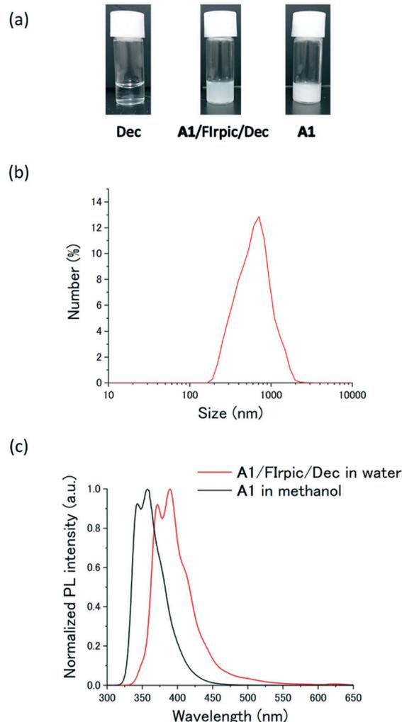
**Fig. 2** (a) Photographs of Dec ([Dec] = 80 mM), **A1**-Firpic-Dec ([**A1**] = 10 mM, [Firpic] = 100 μM, [Dec] = 80 mM), and **A1** ([**A1**] = 10 mM) in water. (b) DLS profile of **A1**-Firpic-Dec in water ([**A1**] = 10 mM, [Firpic] = 100 μM, [Dec] = 80 mM). (c) Fluorescence spectra of **A1** in methanol (black, [**A1**] = 0.25 mM,  $\lambda_{\text{ex}}$  = 241 nm) and **A1**-Firpic-Dec in water (red, [**A1**] = 10 mM, [Firpic] = 100 μM, [Dec] = 80 mM,  $\lambda_{\text{ex}}$  = 280 nm).
