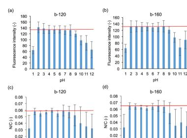
Fig. 5 Results of fluorescence intensity of rhodamine 6G on (a) b-120 and (b) b-160 after pH treatment. Red line shows fluorescence without pH treatment. Results of N/C calculation from XPS measurement on (c) b-120 and (d) b-160 surfaces after pH treatment. Red line shows N/C without pH treatment.
