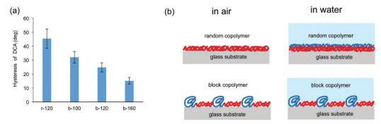
Fig. 3 (a) Hysteresis of DCA for each copolymer and (b) illustration of possible polymer structures of coated films on the glass substrate under air and water conditions
