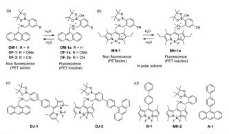
Fig. 1 Proposed mechanisms of PET-type fluorescent sensors (a) OM-1, OF-1, OF-2 and (b) MH-1 for the detection of water in a solvent. Chemical structures of (c) PET/FRET-type fluorescent sensors DJ-1 and DJ-2, (d) BODIPY derivative B-1, PET-type BODIPY MH-2 and anthracene derivative A-1.
