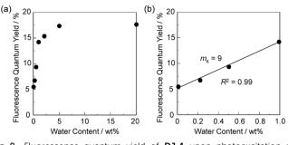
Fig. 8 Fluorescence quantum yield of **DJ-1** upon photoexcitation at 367 nm as a function of water content (a) below 20 wt% and (b) at 1.0 wt% in acetonitrile.
