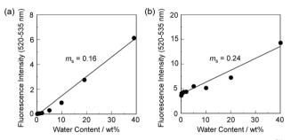
Fig. 7 Fluorescence peak intensity at 520–535 nm of (a) **MH-2** ( $\lambda^{ex}$  = 367 nm) and (b) **DJ-2** ( $\lambda^{ex}$  = 367 nm) as a function of water content below 40 wt% in acetonitrile.
