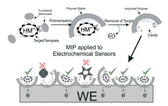
Fig. 4 Schematic representing MIPs applied to electrochemical sensor
