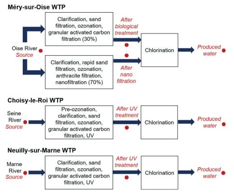
Fig. 1 Treatment processes at the three studied water treatment plants (WTP), with the sampling locations indicated in red.
