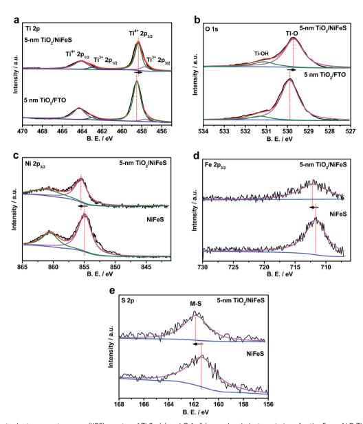
Fig. 4 X-ray photoelectron spectroscopy (XPS) spectra of Ti 2p (a) and O 1s (b) core-level photoemissions for the 5 nm ALD TiO<sub>2</sub> grown on the NiFeS and FTO substrates, and XPS spectra of Ni 2p (c), Fe 2p (d), and S 2p (e) core-level photoemissions comparing the 5 nm  $TiO_2/NiFeS$  and bare NiFeS samples (blue represents the background. Black represents the raw data. The other colours represent fitting curves. The XPS measurement error for binding energies is below 0.03 eV).
