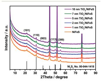
Fig. 1 X-ray diffraction (XRD) patterns of NiFeS nanosheets: bare sample and samples with 1, 2, 5, 7, and 10 nm of atomic layer deposition (ALD)  ${\rm TiO_2}$  coating.
