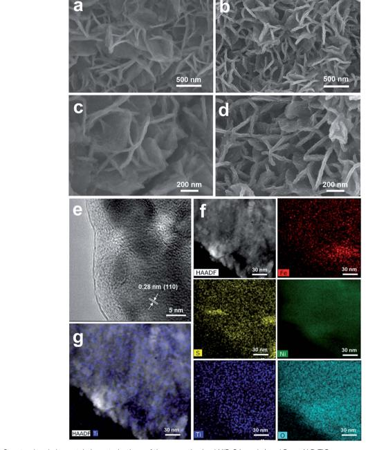
Fig. 3 Structural and elemental characterizations of the as-synthesized NiFeS (a and c) and 5 nm ALD  ${\rm TiO_2}$  grown on the NiFeS nanosheets by scanning electron microscopy (SEM) (b and d), and the high-resolution transmission electron microscopy (HRTEM) image (e), high-angle annual dark-field scanning transmission electron microscopy (HAADF-STEM) image, and energy dispersive X-ray spectroscopy (EDX) elemental mapping images of the 5 nm  ${\rm TiO_2/NiFeS}$  structure (f and g).
