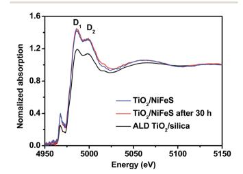
Fig. 6 Comparison of Ti K-edge X-ray absorption near edge structure (XANES) data collected on the as-prepared TiO<sub>2</sub>/silica and 5 nm TiO<sub>2</sub>/ NiFeS nanosheets attached to Ni foam, before and after 30 hours of HER operation.
