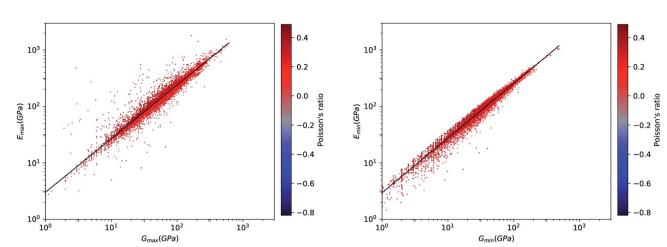
Fig. 8 Plot of extremal values of Young's modulus *versus* shear modulus for 11 764 inorganic compounds, in log-log scale. Left: maximal values; right: minimal values. Poisson's ratio is indicated by color scale. The black lines indicate the linear fit of data:  $\log_{10}(E_{\text{max}}) = 0.95 \log_{10}(G_{\text{max}}) + 0.48 (R^2 = 0.61, \text{ left})$  and  $\log_{10}(E_{\text{min}}) = 0.97 \log_{10}(G_{\text{min}}) + 0.47 (R^2 = 0.96, \text{ right})$ .
