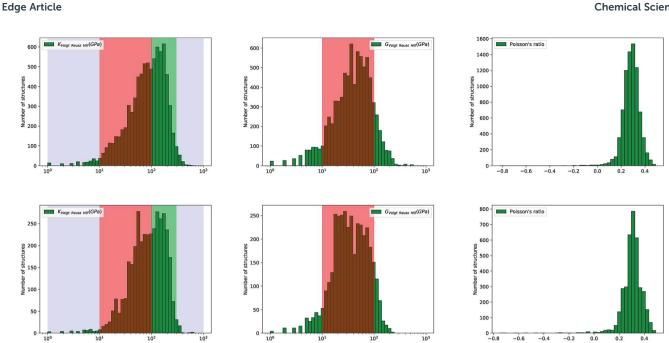
Histograms of  $log(K_{VRH})$ ,  $log(G_{VRH})$ , and Poisson's ratio v for 8050 synthesized (top) and 3714 hypothetical (bottom) inorganic compounds.
