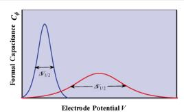
Fig. 2  $C_{\phi}$  vs. electrode potential profiles for an electrosorption process involving a zero (blue) and a positive (red) g value, *i.e.*, for lateral repulsion. Adapted from Fig. 10.1 in ref. 10 p. 228, with permission.
