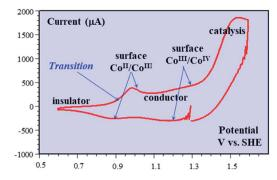
Fig. 5 Cyclic voltammetry current–potential responses (potential:  $1.29 \rightarrow 0.59 \rightarrow 1.59 \rightarrow 1.29$  V vs. SHE) at 8 V s<sup>-1</sup> of a 39 nm cobalt oxide deposited (CoP<sub>i</sub>) film in the presence of 0.2 M potassium phosphate (KP<sub>i</sub>) at pH = 7. Adapted from Fig. 2 in ref. 18 with permission.
