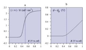
Fig. 9 (a) Forward CV scan for with  $C_d = 2.55 \text{ mF cm}^{-2}$  (i.e. capacitance of a 40 nm CoP<sub>i</sub> film),  $F^2N/RT = 20 \text{ mF cm}^{-2}$  (i.e.  $N = 8 \times 10^{20}$ cm<sup>-3</sup> for a 40 nm film),  $E^{0,ap} - \Delta E^{0}/2 + \phi_{S} = 0.5 \text{ V}$  (dashed vertical line), T = 298 K. (b) Evolution of the film inner potential. Adapted from Fig. 5 in ref. 19 with permission.
