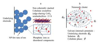
Fig. 8 (a) Structural sketch of cobalt oxide electrodeposited films. (b) Scheme of the various phases considered in the electrochemical description of a cobalt oxide electrodeposited. Adapted from Fig. 4 in ref. 18 with permission.
