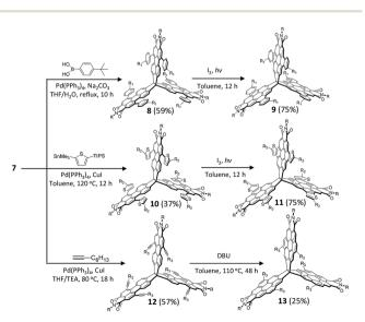
Scheme 2 Synthesis of quasi- $D_{3h}$  symmetric nanostructures based on **6**.
