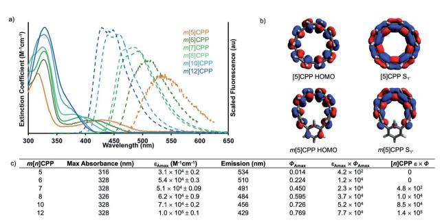
Fig. 3 (a) Absorbance and emission spectra of m[n]CPPs; (b) HOMO (left) and  $S_{1'}$  (right) orbital depiction of [5]CPP and m[5]CPP, demonstrating change in orbital symmetry. Calculated using CAM-B3LYP/STO-3G level of theory; (c) absorbance, extinction coefficient ( $\varepsilon$ ), emission and quantum yield ( $\Phi$ ) of m[5]-m[8]-, m[10]- and m[12]CPP and brightness comparison of m[n]CPPs and m[n]CPPs.
