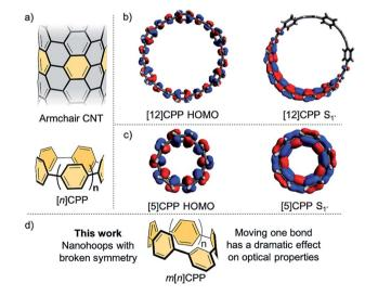
Fig. 1 (a) Structure of an armchair carbon nanotube (CNT) and its relation to [n]cycloparaphenylenes; (b) HOMO (left) and excited state (right)  $S_{1'}$  orbitals of [12]CPP and (c) HOMO (left) and excited state (right) S<sub>1'</sub> orbitals of [5]CPP. Orbitals have been calculated using CAM-B3LYP/STO-3G level of theory. (d) meta[n]CPPs with broken symmetry in this work.
