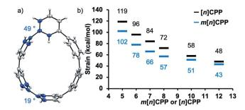
Fig. 2 (a) Molecular structure of m[6]CPP determined by X-ray crystallography (thermal ellipsoids shown at 50% probability). (b) Calculated strain using homodesmotic reactions of [n]CPPs (black) and m[n] CPPs (blue) at B3LYP/6-31G(d,p) level of theory.
