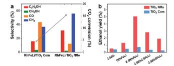
Fig. 3 (a) The  $CO_2$  conversion (grey) and product selectivity of 2.5 wt% RhFeLi/TiO<sub>2</sub> NRs and 2.5 wt% RhFeLi/TiO<sub>2</sub> Com. (b) The ethanol yield of the Rh-based catalyst supported on TiO<sub>2</sub> NRs and TiO<sub>2</sub> Com.
