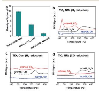
Fig. 4 (a) The peak area of hydroxyls in FTIR normalized by  $S_{\rm BET}$  ( $\times 10^3$ ) on 2.5 wt% RhFeLi/TiO $_2$  NRs, 2.5 wt% RhFeLi/TiO $_2$  Com and 2.5 wt% RhFeLi/TiO $_2$  NRs-CO. (b) CO-TPD profiles of 2.5 wt% RhFeLi/TiO $_2$  NRs. Pretreatment: H $_2$  reduction at 400 °C. (c) CO-TPD profiles of 2.5 wt% RhFeLi/TiO $_2$  Com. Pretreatment: H $_2$  reduction at 400 °C. (d) CO-TPD profiles of 2.5 wt% RhFeLi/TiO $_2$  NRs. Pretreatment: CO reduction at 350 °C.
