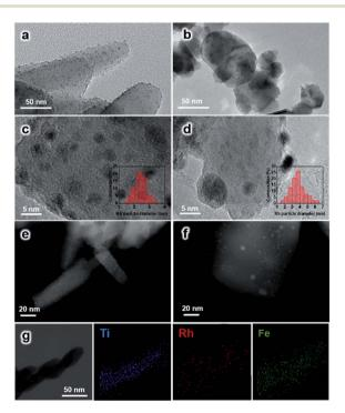
Fig. 1 (a and b) TEM; (c and d) HRTEM images, particle size distributions (inset figures) and (e and f) HAADF-STEM images of catalysts after reaction. (a, c and e) 2.5 wt% RhFeLi supported on  $\rm TiO_2$  NRs and (b, d and f) 2.5 wt% RhFeLi supported on  $\rm TiO_2$  Com. (g) STEM-EDS elemental mapping of 2.5 wt% RhFeLi supported on  $\rm TiO_2$  NRs.
