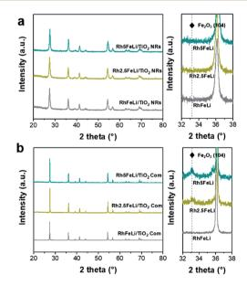
Fig. 2 (a) XRD spectra of 2.5 wt% RhFeLi/ $TiO_2$  NRs with different Fe loadings. (b) XRD spectra of 2.5 wt% RhFeLi/ $TiO_2$  Com with different Fe loadings. The figures on the right of (a) and (b) show the enlarged XRD patterns.
