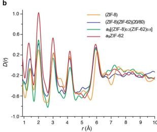
Fig. 4 (a) Structure factors S(q) of (ZIF-8)(ZIF-62)(20/80),  $a_g[(ZIF-8)_{0.2}(ZIF-62)_{0.8}]$  and ZIF-8, alongside that of  $a_gZIF-62$  from a previous publication.<sup>46</sup> (b) Corresponding X-ray pair distribution functions D(r).
