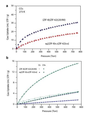
Fig. 7 (a)  $\rm CO_2$  isotherm at 273 K and (b)  $\rm O_2$  and  $\rm CH_4$  at 273 K isotherms for zinc based samples. Closed symbols represent adsorption isotherms and open symbols represent desorption isotherms.
