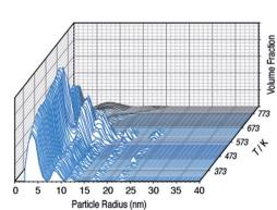
Fig. 3 Temperature resolved diffraction of (a) WAXS profile of (ZIF-8)(ZIF-62)(20/80) and (b) volume fraction distributions of (ZIF-8)(ZIF-62)(20/80).
