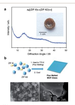
Fig. 2 (a) Powder X-ray diffraction pattern of the glass formed after quenching from 773 K, and (inset) optical image. (b) Schematic of flux melted glass formation and SEM images of (left) (ZIF-8)(ZIF-62)(20/80) and (right)  $a_g[(ZIF-8)_{0.2}(ZIF-62)_{0.8}]$ .
