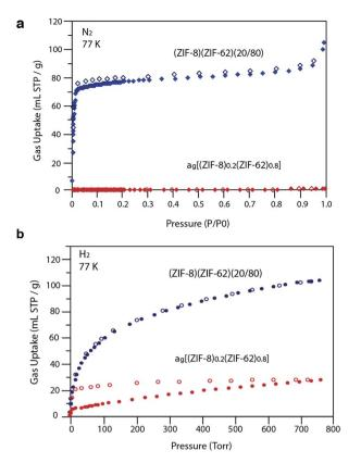
Fig. 6 (a)  $N_2$  at 77 K and (b)  $H_2$  at 77 K gas isotherms for the zinc-based crystalline mixtures and glasses. Closed symbols represent adsorption isotherms and open symbols represent desorption isotherms.
