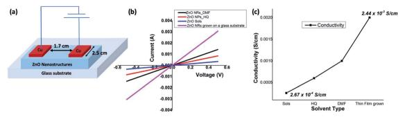
Fig. 7 (a) A schematic diagram of a test device used for I-V characterization; (b) I-V graphs of ZnO nanostructures; and (c) the electrical conductivities of solution formed nanorods and nanoparticles comparing with the electrical conductivity of sols and solvothermal grown nanorods from ZnO sols-casted glass substrate.
