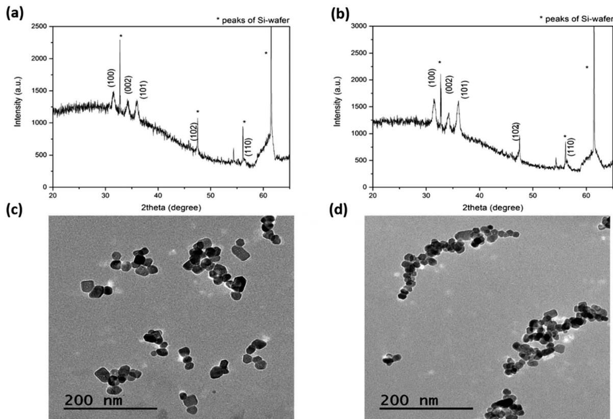
Fig. 1 Structural and morphological characterization: XRD patterns for (a) ZnO and (b) ZnO-NH<sub>2</sub> NCs; TEM micrographs of (c) ZnO and (d) ZnO-NH<sub>2</sub> NCs.
