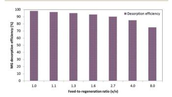
Fig. 14 Effect of different feed-to-regeneration ratios (v/v) on the desorption efficiency of malachite green (MG) dye (water as regeneration solution; adsorbent dosage = 0.02 g L<sup>-1</sup>, MG initial concentration ( $C_{\rm o}$ ) = 25 mg L<sup>-1</sup>; replication = 3; standard deviation:  $\pm$  1.59).
