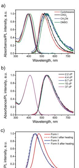
Fig. 4 Steady-state optical data: absorption and PL spectra of BFMPT in different organic solvents (a) and DMSO:glycerol mixtures of different viscosity (2.2–37 cP) (b); PL spectra of BFMPT crystals measured by
