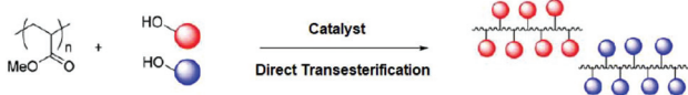
Fig. 14 Transesterification-based synthetic strategy to functional polyacrylates. Reproduced from ref. 136 with permission from WILEY-VCH Verlag GmbH & Co., copyright [2017].
