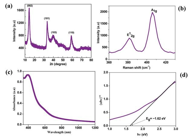
Fig. 1 (a) X-ray diffraction pattern of MoS<sub>2</sub>. (b) Raman spectrum of MoS<sub>2</sub>. (c) Absorption spectrum and (d) Tauc plot of MoS<sub>2</sub>.
