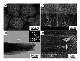
Fig. 6 (a and b) SEM, (c) TEM, and (d) HRTEM images of rutile TiO<sub>2</sub> nanorod arrays prepared at 150 °C on Ti foil for 20 h. The inset in (c) is the corresponding SAED pattern. Adapted with permission from ref. 64. Copyright 2012 Royal Society of Chemistry.
