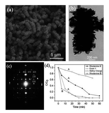
Fig. 18 (a) SEM image of caterpillar-like AgIn(WO<sub>4</sub>)<sub>2</sub> mesocrystals. (b) TEM image of an individual caterpillar-like particle. (c) Corresponding SAED pattern. (d) Photocatalytic degradation of different organic dyes under 300 W Xe lamp irradiation with AgIn(WO<sub>4</sub>)<sub>2</sub> mesocrystals. Adapted with permission from ref. 110. Copyright 2010 Royal Society of Chemistry.
