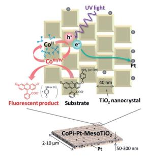
Fig. 20 Schematic illustration of the photogenerated charge transfer on the surface of CoPi/Pt/TiO<sub>2</sub> mesocrystal. Adapted with permission from ref. 117. Copyright 2014 Royal Society of Chemistry.
