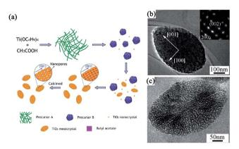
Fig. 3 (a) Schematic illustration of a tentative mechanism for the additive-free synthesis of porous anatase TiO2 mesocrystals. (b) A lowmagnification TEM image of a single spindle. Inset shows the corresponding SAED pattern. (c) A high-magnification TEM image of a porous particle. Adapted with permission from ref. 44. Copyright 2011 American Chemical Society.
