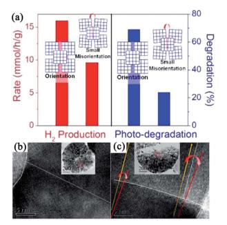
Fig. 4 (a) Schematic illustration of disordered and ordered aggregations of TiO2 nanoparticles and their corresponding photocatalytic activities. (b) HRTEM image of TiO2 mesocrystal with ordered orientation. (c) HRTEM image of TiO<sub>2</sub> mesocrystal with misorientation (crystal lattice mismatch). Adapted with permission from ref. 53. Copyright 2015 American Chemical Society.
