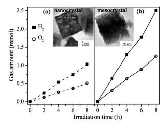
Fig. 14 Photocatalytic water splitting for hydrogen and oxygen generation. (a) Nanocrystals (dashed line) and (b) NaTaO<sub>3</sub> mesocrystals (solid line). Adapted with permission from ref. 101. Copyright 2013 Elsevier.
