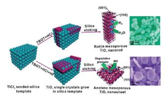
Fig. 5 Schematic illustration of the synthesis pathways of rutile TiO<sub>2</sub> mesocrystals and anatase TiO<sub>2</sub> mesocrystals using silica templates by a hydrothermal method. Adapted with permission from ref. 61. Copyright 2013 American Chemical Society.
