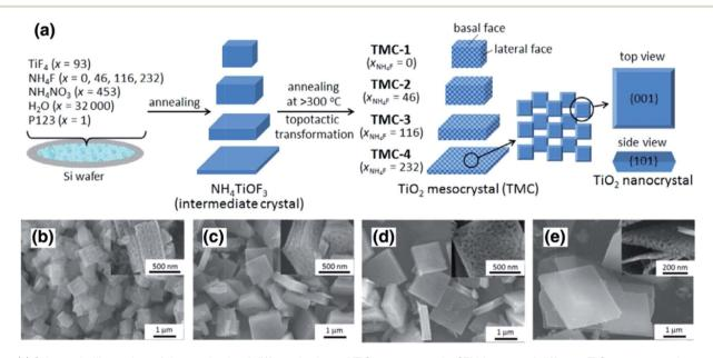
Fig. 1 (a) Schematic illustration of the synthesis of differently shaped  $TiO_2$  mesocrystals. SEM images of different  $TiO_2$  mesocrystals prepared with x (molar ratio of NH<sub>4</sub>F) = 0 (b), 46 (c), 116 (d), and 232 (e). Insets display the corresponding high-magnification SEM images. It can be found that the thickness size of the as-synthesized particles gradually reduced along with an increase in the amount of  $NH_4F$ . Adapted with permission from ref. 26. Copyright 2016 Elsevier.
