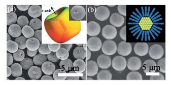
Fig. 7 (a) SEM image of ZnO apple-like structures. Adapted with permission from ref. 78. Copyright 2011 Nature Publishing Group. Inset shows the corresponding schematic illustration and a typical particle. Adapted with permission from ref. 77. Copyright 2009 American Chemical Society. (b) SEM images of the ZnO mesocrystal microspheres. Inset is the corresponding schematic illustration. Adapted with permission from ref. 78. Copyright 2011 Nature Publishing Group.
