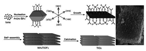
Fig. 2 Schematic illustration of the formation of layered TiO<sub>2</sub> mesocrystals. Adapted with permission from ref. 41. Copyright 2011 Wiley-VCH Verlag GmbH & Co
