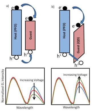
Fig. 1 Schematic energy diagram and electroluminescence spectrum of (a) blend of large band gap organic host and an organic dye resulting in severe electron trapping. (b) Blend of large band gap organic host and an inorganic QD, leading to electron trapping and charging effects that enhance hole capture
