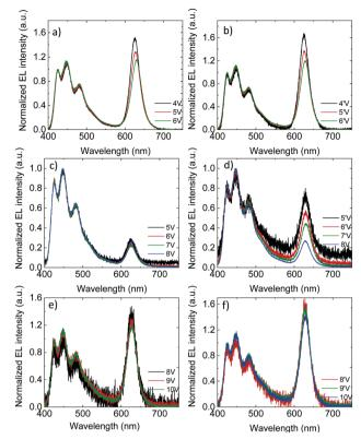
Fig. 3 Voltage dependence of normalized EL spectra for PLED with 100 nm PFO:3% oa-QD/PS blend active layer (a) first up-scan and (b) consecutive down-scan. Voltage dependence of normalized EL spectra for PLED with 100 nm PFO:3% QD/PS-hybrid blend active layer (c) first upscan and (d) consecutive down-scan, (e) fifth up-scan and (f) corresponding down-scan
